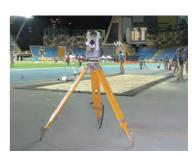
Optical distance measuring equipment DM-400
