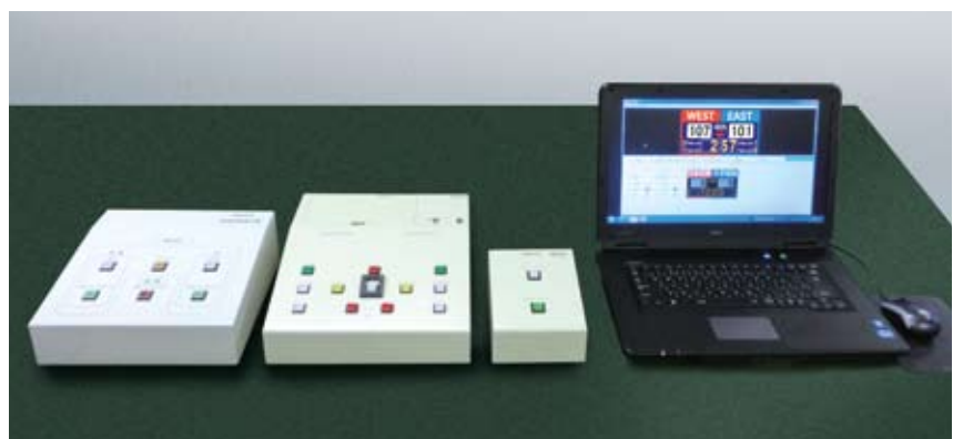
From left, Budo Time Operation Board, Game Operation Board, Time Operation Board, and Team Name/Score Input Device
